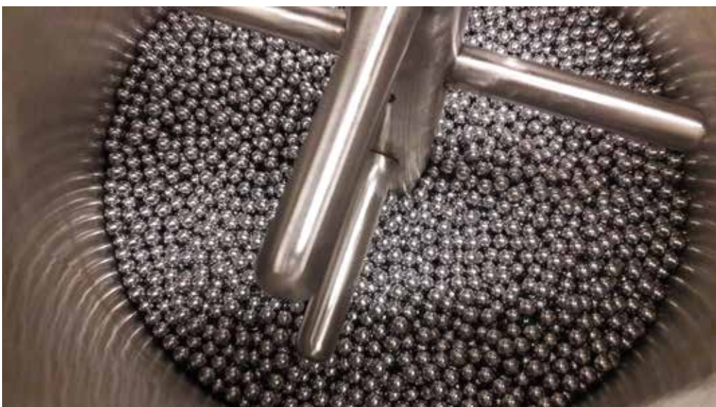
Figure 6 Refining / homogenisation plant with balls
